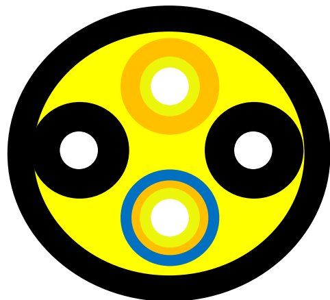
7.0mm LSZH Jacket with Two 2.0mm SM or MM Fibers & Two Stuffing Cable
